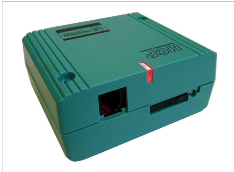
Figure 9. Red status LED flashing on M485 Terminal
