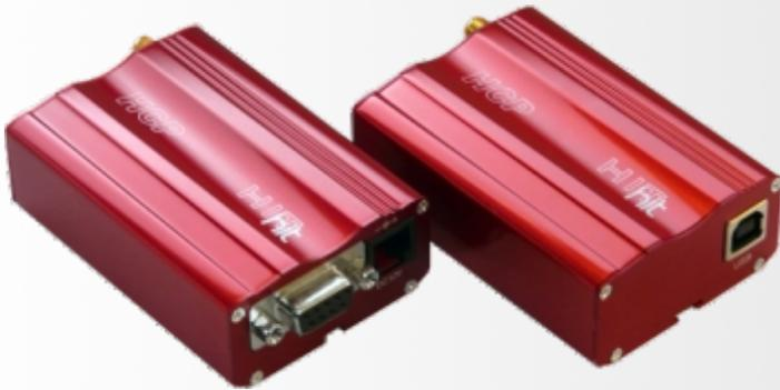
This is easy-to-use quad band GSM/GPRS modem that enables data, fax and SMS applications.
