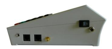
Picture of the connectors from left to right: for a cash drawer, PC, Bar Code Scanner, GSM antenna and power supply DC.
