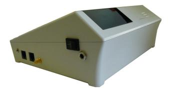
ECR HCP MECHARE uses power supply of 24V DC and also has a backup battery power.
