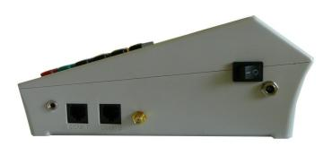
Picture of the connectors from left to right: for a cash drawer, PC, Bar Code Scanner, GSM antenna and power supply.
